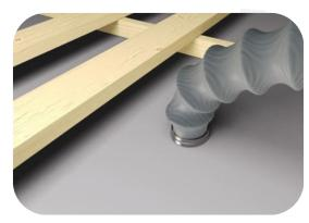
Attach ducting onto the air valve mounting ring
